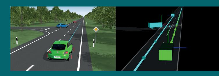
Exemplary driving functions were developed in the IMAGinE project that not only focus on a single vehicle, but also involve multiple vehicles interacting via V2X communication for joint solution finding.
